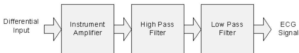
Fig. 3. ECG amplifier block diagram
