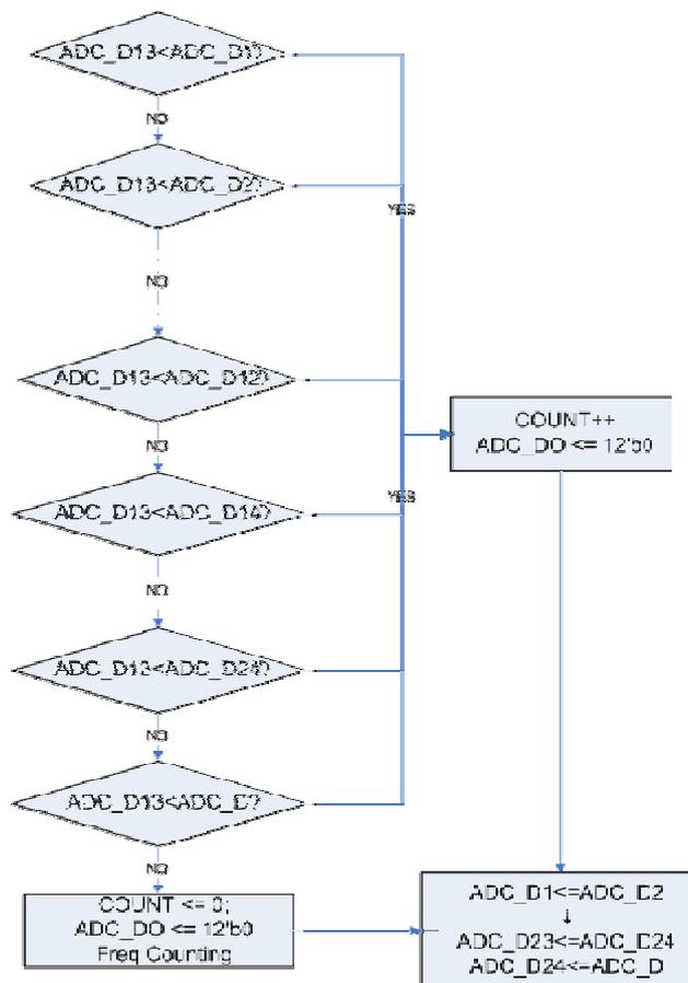
Fig. 11. Maximum point flowchart
