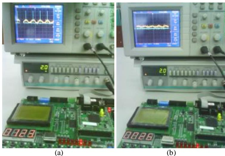
Fig. 16. (a) 2 Hz, 100 mV input, display: 123 (b) 2 Hz, 80 mV input, display: 26
