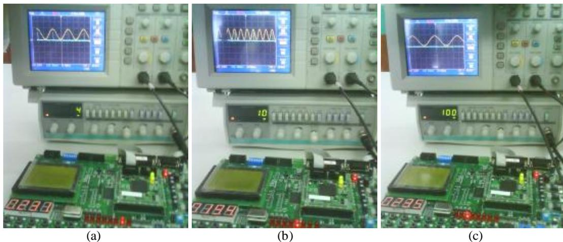
Fig. 15. (a) 4 Hz input, display: 231 (b) 10 Hz input, display: 194 (c) 100 Hz input
