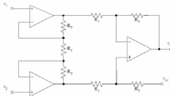
Fig. 5. Instrumentation amplifier circuit diagram
