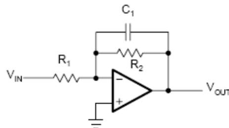
Fig. 7. First order inverting active low pass filter
