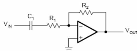
Fig. 6. First order inverting active high pass filter
