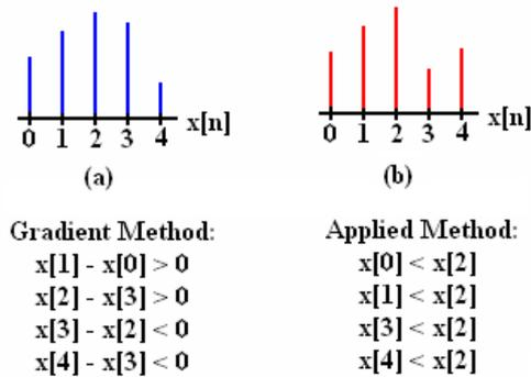
Fig. 12. Two different maximum point methods
